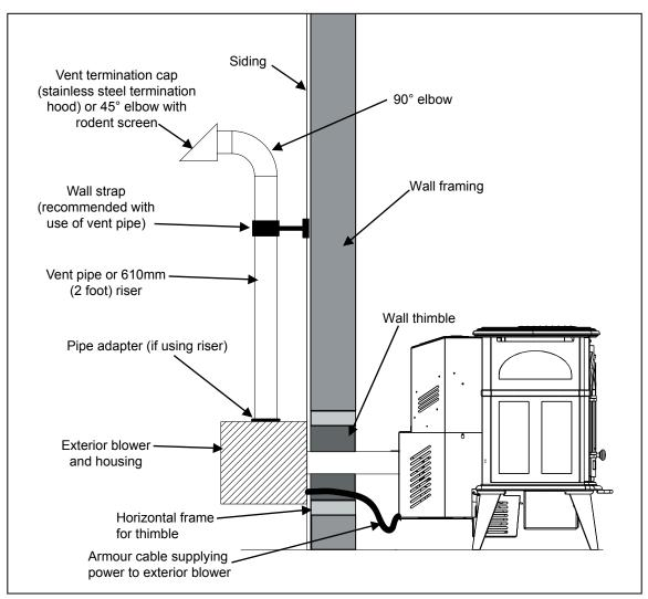
Figure 19: Exhaust Blower Installation; Horizontal Termination.
